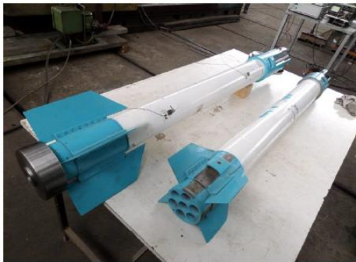
Fig. 1 Positioning the strain gauges on the first portion of the rocket
