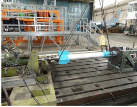
Fig. 5 Positioning the rocket launcher
