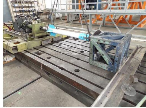
Fig. 6 Fixing the rocket launcher on the testing stand
