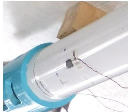
Fig. 2 The strain gauge on the first portion of the rocket (detail)
